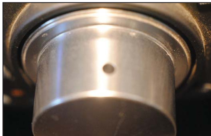
Photo D. A tiny hole in the tuning knob contains a set screw which needs to be loosened.
