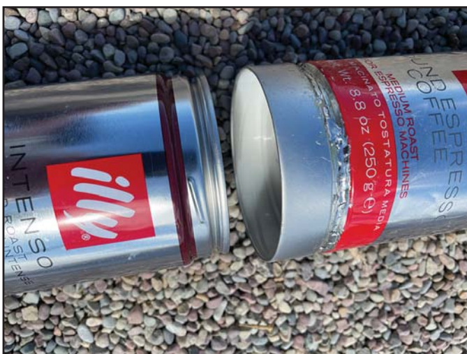
Photo C. The screw-on lid of each of the Illy coffee cans is soldered to the bottom of the can with the screw-on section facing down.
