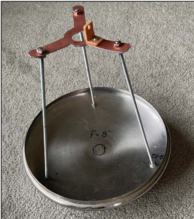
Photo A. Nine-inch dish with wide beamwidth
