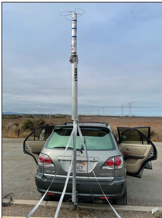
Photo F. The antenna may look funny, but it has a low SWR, broad bandwidth and works well!
