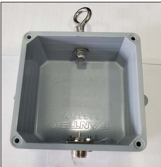
Photo A. Unun enclosure with hardware
