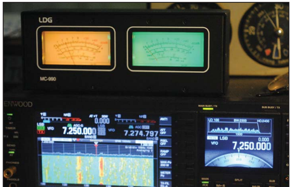
Photo K. The limited-production LDG dual analog color meter set is “plug and play” with most larger rigs that have a “meter” jack on the rear panel. The meters will give you a much larger display of various parameters.
