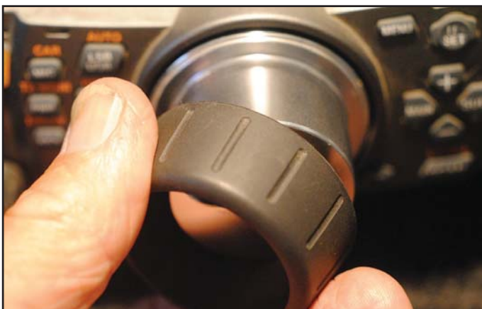
Photo J. Once you've put the knob back on the shaft and tightened the set screw, you can slide the rubber ring back on and you should be good for a few million more spins!
