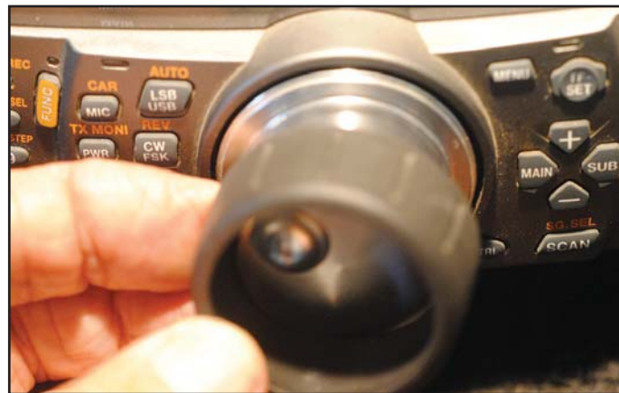
Photo C. Once you've loosened it up by hand, the ring can be gently pried off.
