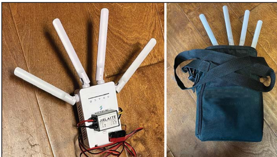
Photo G: One of the relay stations. Contents include a 7-amp-hour 12VDC battery, a 12-5VDC converter (required by the relay station), a 10-foot-long 120VAC extension cord, a 2-foot-long 12VDC power cable, and four antennas:
